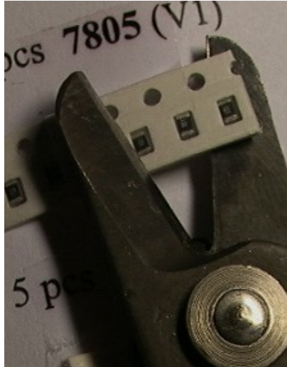
Illustration 3: Cut components as you need them to prevent loosing any of them
